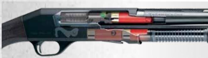
Near the end of the recoil cycle, chamber pressure drops to a safe level and the gun's rearward motion slows. The heavy inertia spring then thrusts the bolt assembly rearward, unlocking the rotating bolt head, extracting the spent shell from the chamber and pulling it against the ejector.
