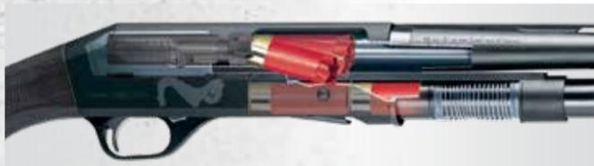
As the empty shell exits the receiver, the energy of the moving bolt assembly re-cocks the hammer and compresses the recoil spring on the magazine tube. The recoil spring then thrusts the bolt assembly forward lifting the on-coming shell into position and chambering a fresh cartridge. The gun is ready to fire again...in a fraction of a second!
